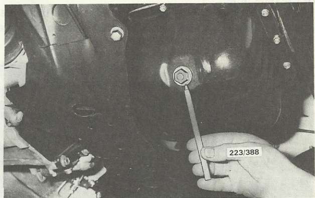
Location of engine sump drain plug with splash guard removed.
