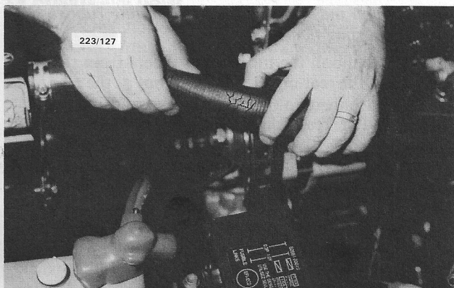
Check for leaking and damaged radiator hoses and welch plugs.
