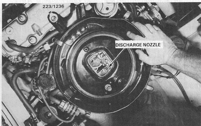
Check for discharge of fuel at the carburettor accelerator pump discharge nozzle.
