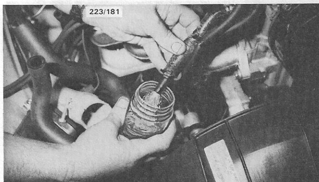
Checking for fuel at the carburettor inlet pipe.
