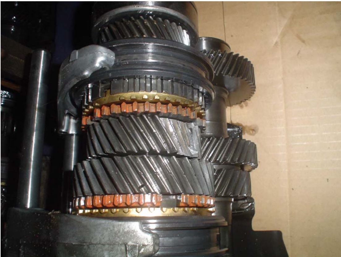
Figure 21: W58 with 4 th gear engaged (steel plate; NOTE: this is Norbie's gearbox Ex JZA80 with 3 rd gear damage)
